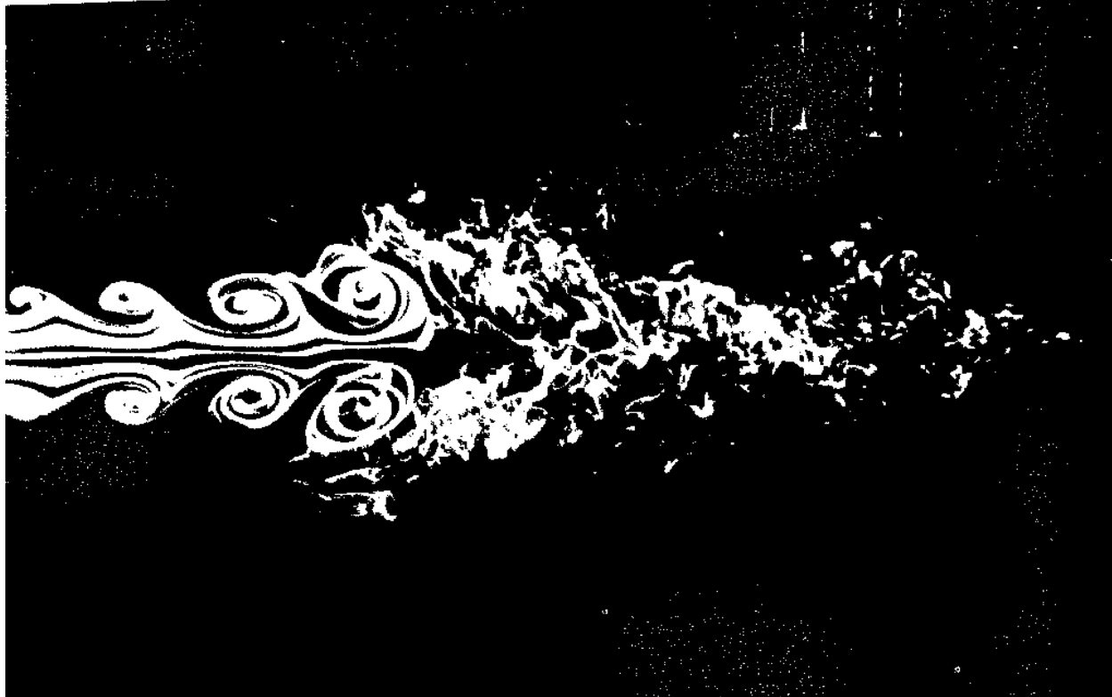
Figure 9: Instability of an axisymmetric jet (Drubka and Nagib).
