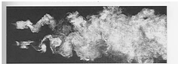
Fig. 1.10. Wake behind two identical cylinders at R = 1800 . Courtesy R. Dumas.
